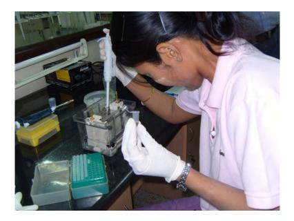
Loading the DNA sample in the wells of casting gel
